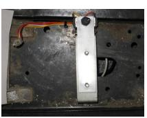
9.) Slide the contactor back into position and reinstall the contactor nuts (11mm socket) as shown in Figure 13.
